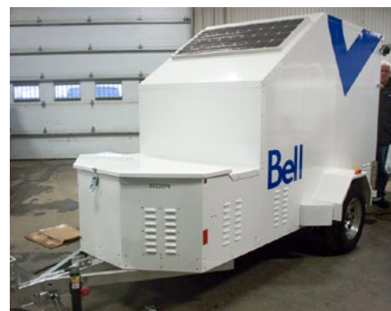
Bell trailer which has an 80-watt solar panel that enables recharging of a 12-volt battery.
